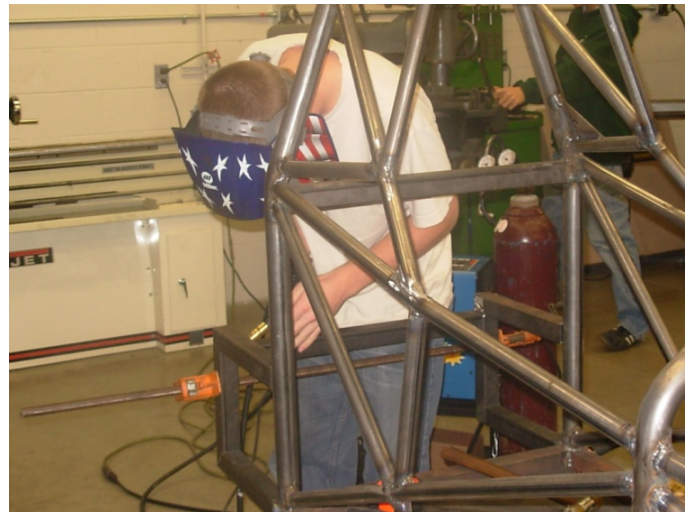
Matt welding the engine mount
